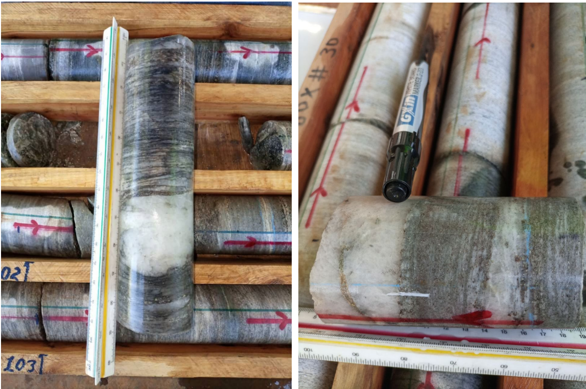
Figure 1: Drill core from Hole 1 (BBDD001), showing intervals of highly altered host rocks and quartz veining, both with significant visible sulphide mineralisation (pyrite, chalcopyrite, pyrrhotite). Left: ca. 101m Right: ca. 106m
