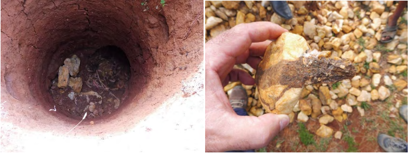
FIGURE 12: ARTISANAL MINING PIT (LEFT). BRECCIATED QUARTZ FROM ARTISANAL PIT (RIGHT)
