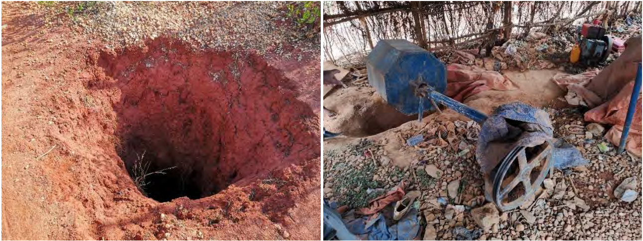
FIGURE 6: BURRI KARROO ARTISANAL PIT (LEFT) AND SMALL MILL TO FREE GOLD FROM EXTRACTED QUARTZ GRAVELS (RIGHT)
