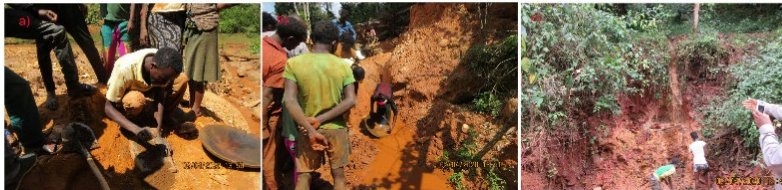
Plate 1: Locals working for gold in the Ad56 a) crushing washout rock fragments for second round panning at BGR0032 sampling site, b) panning the crushed rock, c) preparing channel for ground sluicing.
